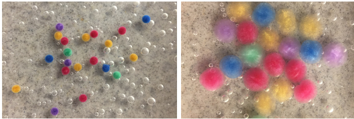
Figure 4. The left shows the original size of the hydrogel and the right shows when they are swollen into 80% of its full size.
